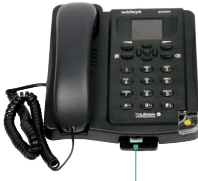
SIM Card with gold contact facing up
